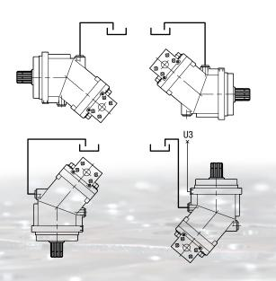
In installations where the position of the pump is above the tank, ensure the drain line is always underneath the fluid level tank.
